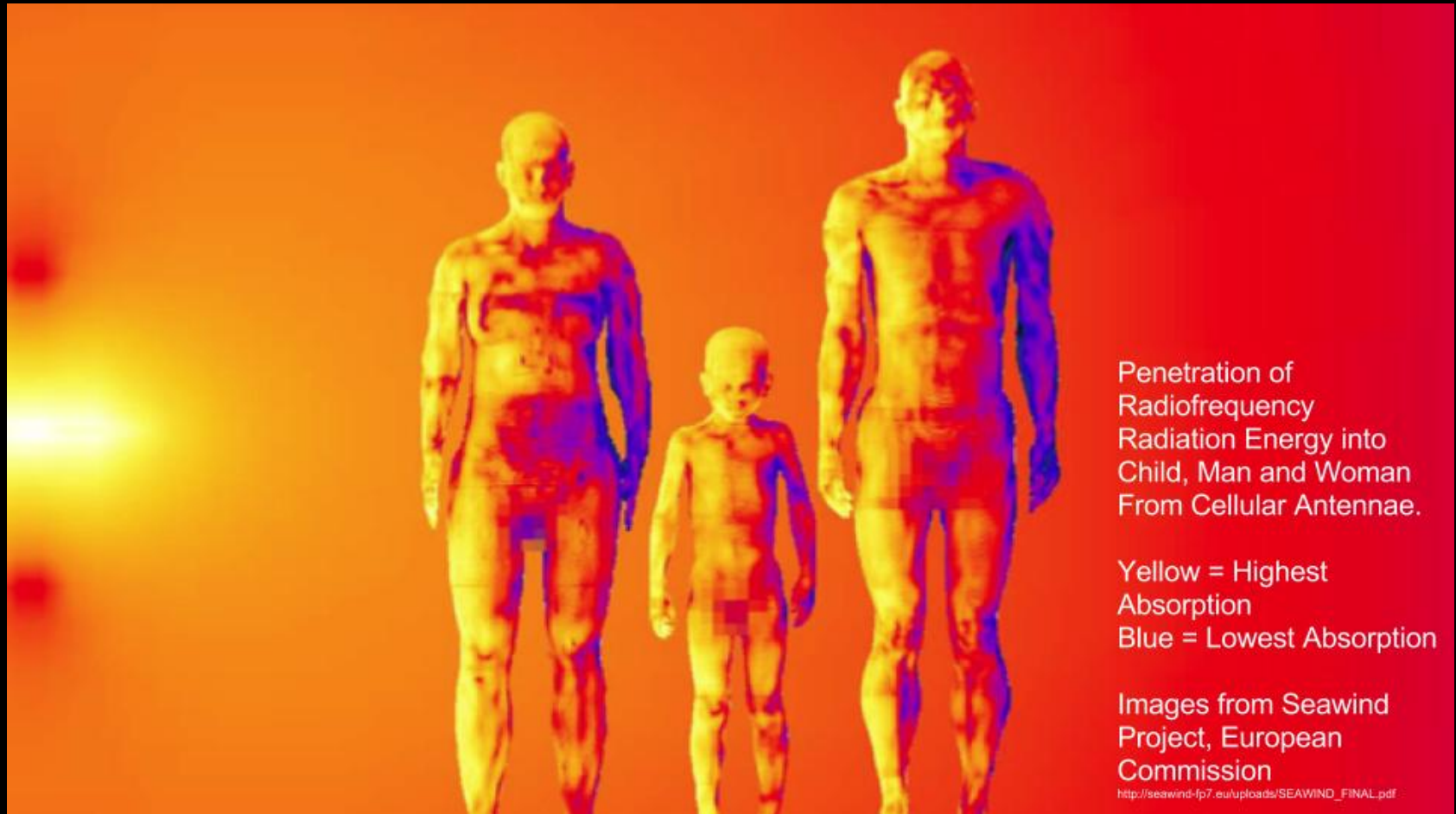
Image of the simulation of far field radiation penetration into differently aged humans. Seawind Project, EU Commission
