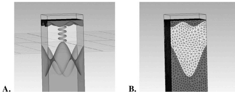
Figure 2 The 3-layer skin model. The simulation is conducted over the (a) unit cell using (b) tetrahedral mesh. Periodic boundary conditions extend the model into the surrounding space [3,4].
