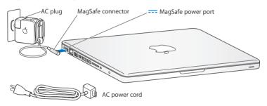
To extend the reach of your power adapter, replace the AC plug with the AC power cord. First pull the AC plug up to remove it from the adapter, and then attach the included AC power cord to the adapter, making sure it's seated firmly.
