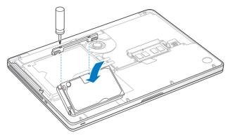
9 Replace the bracket and tighten the screws.
