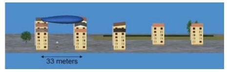
**Figure 5.** The compliance distance of a typical roof-mounted base station, calculated for an exposure limit of 0.6 V/m, is 165 meters in the forward direction. $^5$
