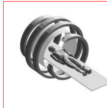
The apparatus for Nuclear Magnetic Resonance Imaging includes magnets applying a magnetic field and magnetic field gradient (the four narrow rings), and EMR coils (the inner cylinder) [Rubenstein, 1988].
