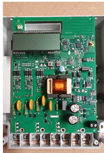
Smart meter with built-in power supply and processor capacity that creates more voltage noise while having less efficient noise filters.
