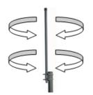
Whip - Antenna that radiates energy equally in all directions. Maintain as much distance as possible from this antenna.
