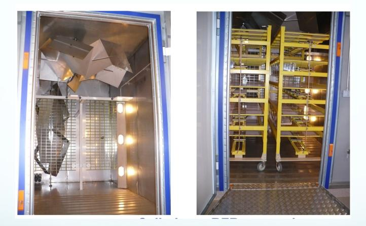
A shielded room from penetrating EMFs containing an excitation antennae and ventilation panels. Field exposures emanate from multiple angles (all directions), while rotating paddles distribute the fields to create a statistically homogeneous electromagnetic environment. No limit on daily exposure time, no comparable historical control.
